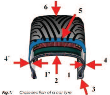
Fig.1: Cross-section of a car tyre showing the main measurement points of the rubber thickness up to the steel mesh: 1, 1' inside at the sidewall 2 inside underneath the tread 3 above the beads 4, 4' outside at the sidewall 5 under-tread thickness 6 tread thickness
